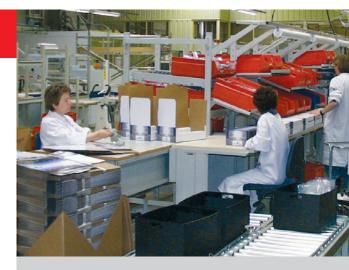
The packing and shipment of products forms an important part of the industrial process. Operation is often automated as production volumes soar. By this stage, all of the required tasks and processes have already been properly designed, and all that is needed is a new, compact, space-saving transfer system. Standard modules are easy to integrate with existing packing equipment, keeping investment costs low.
